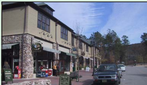
Groundfloor stone pilasters (attached pillars), store-front bays, and canvas awnings are used on these new buildings to break up the facade into a series of vertically oriented bays.
